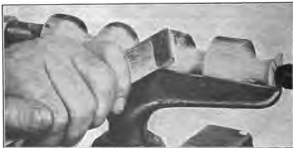
Fig. 54. Turning Bead with Skew Chisel.
